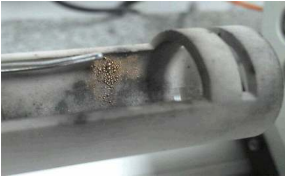
Figure 2. Vaporization of copper inside the dilatometer tube.
