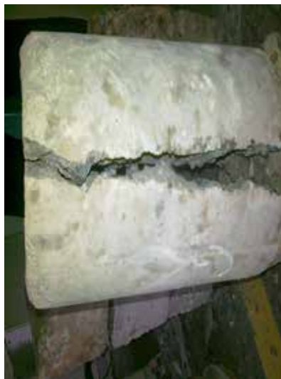
Figure 1: Failure of cylinders
