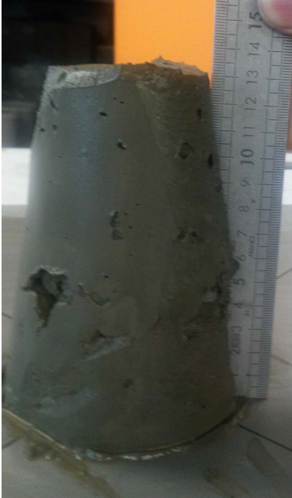
Figure 2.3: A minicone test is performed on the fresh cement paste C985NS015 featuring 1.5% NS at water-to-cement ratio 0.35. The initial height of the minicone is 150mm and the final height is about 130mm : this cement paste does not significantly flow under its own weight.
