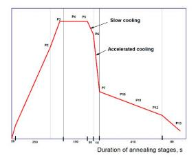
**Figure 1.** Scheme of heat treatment of cold-rolled steels in a continuous annealing unit (CAU): Pi—strip temperatures at the exit from the zones of heating sections (P2, P3), holding (P4, P5), slow cooling (P6), accelerated cooling (P7), overaging (P10, P11, P12) and final cooling (P13).
