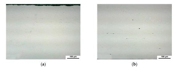
**Figure 2.** Nonmetallic inclusions in the samples of the batches: (**a**) Point and line inclusions (No. 2-2); (**b**) Extended inclusions (No. 2-1).
