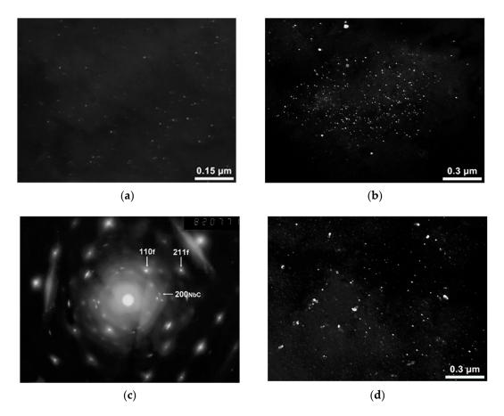
**Figure 7.** Nanosized NbC particles in samples of the batches (TEM): (**a**) No. 1-1; (**b**) No. 2-2; (**c**) No. 2-2; (**d**) No. 2-1. Dark-field images in reflections of nanocarbides (**a**,**b**,**d**) and microdiffraction pattern with marked reflections of NbC and (some) ferrite—f (**c**).
