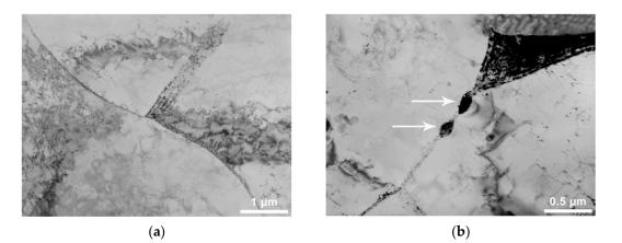
**Figure 5.** Microstructure of samples of the batches (TEM, bright-field images): (**a**) Polygonal ferrite (No. 1-1); (**b**) Cementite precipitation indicated by arrows (No. 2-2).
