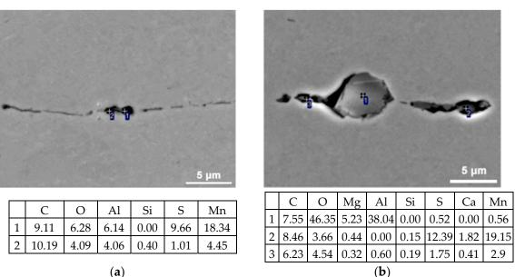
addition of magnesium, the sulfide component is manganese sulfide, sometimes with the addition of calcium. It is important that the composition of inclusions in samples of different rolled products has a similar composition
