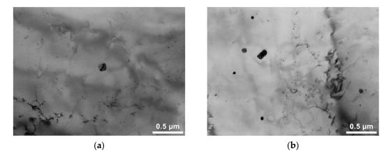
**Figure 6.** Submicron precipitates in samples of the batches (TEM, bright-field images): (**a**) No. 1-1; (**b**) No. 2-2.
