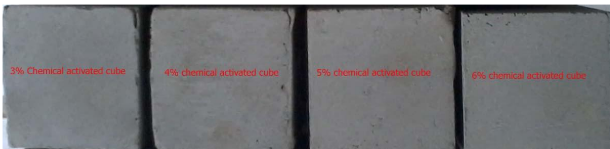
Figure-3: Geopolymer specimens after 60 days atmospheric curing.
