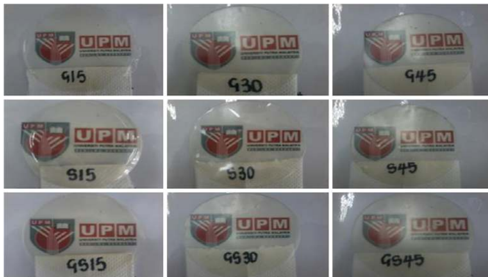
Fig. 2 SPS films prepared using different plasticizer type and concentration
