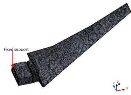
Fig. 5. HIRENASD wing structure finite element mesh
