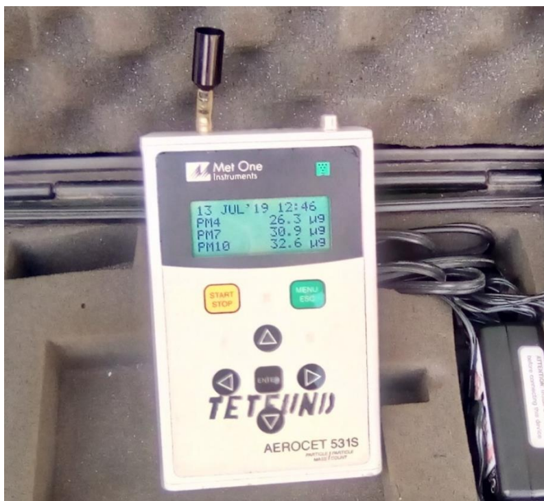
Fig. 3: A Portable Digital Particle Mass/Count Instrument Call Met One Instruments AEROCET 531S
