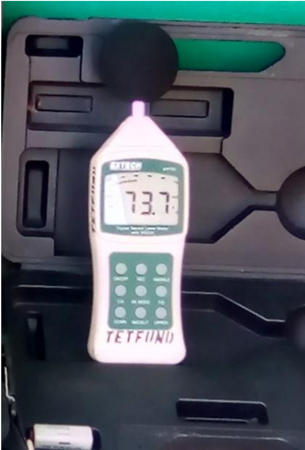
Fig. 5: A Portable Digital Sound Level Meter with RS232 Extech 407750
