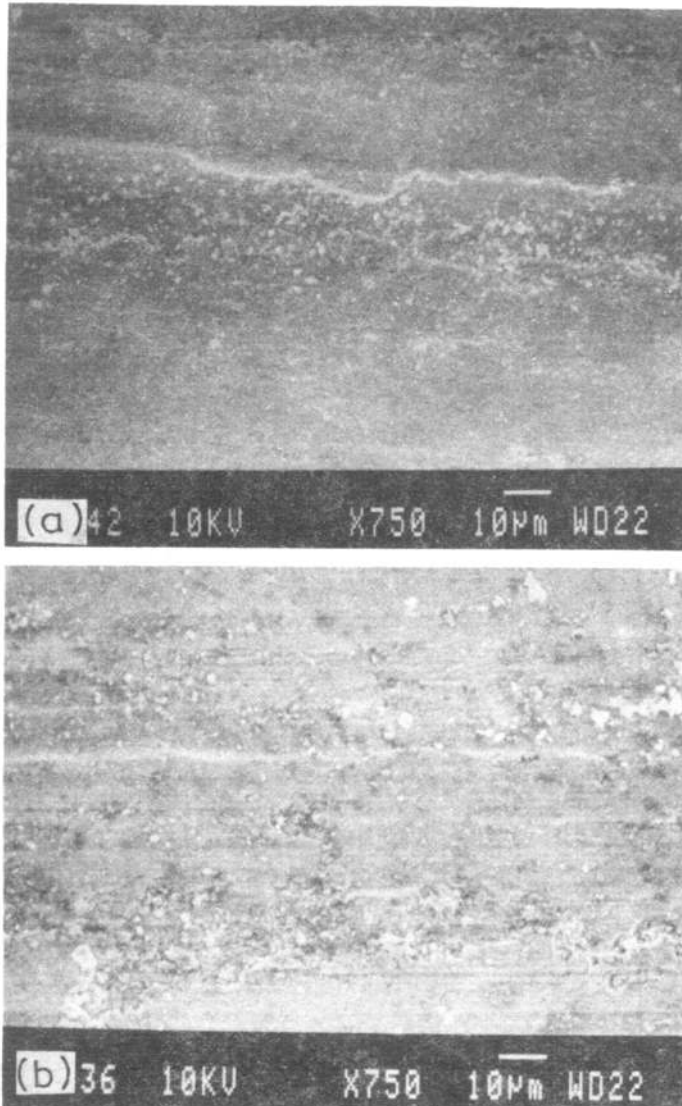
Figure 7. Scanning electron micrograph of worn out surface of specimen prepared from impeller mixed alloy at applied load of (a) 10 N and (b) 30 N.
