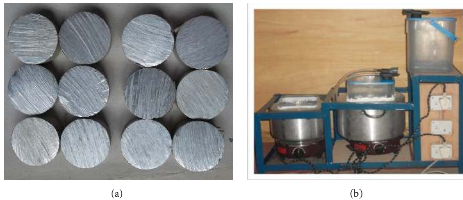
FIGURE 1: (a) Cast aluminium alloy specimen and (b) EN plating bath line [10].
