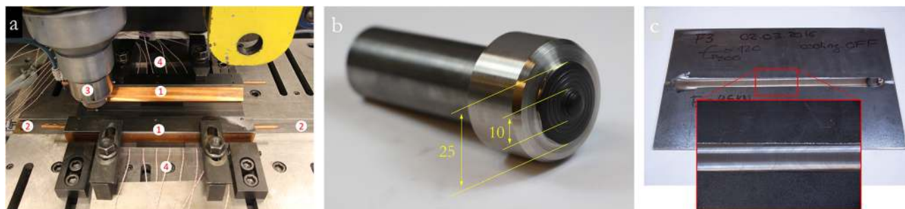
Fig. 1 Welding setup and tool for FSW. a Details of the clamping system and temperature measurement setup including (1) water cooled clamping elements. The average water temperature was \approx 7 °C and the flow was 8 L/min; (2) water cooled anvil; (3) shielding gas nozzle; and (4)
