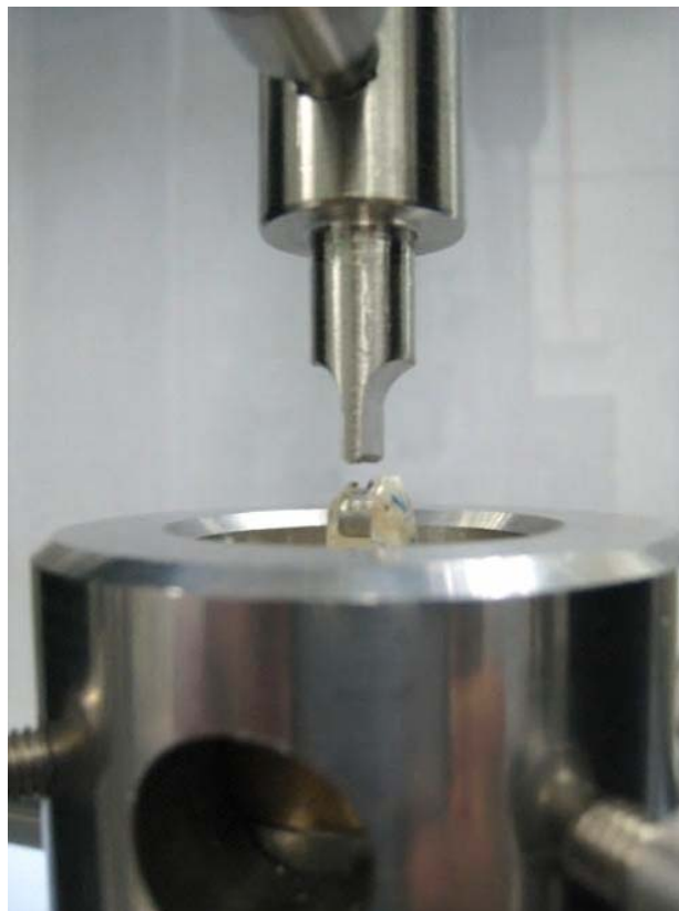
Figure 2. Tooth sample assembled to the universal testing machine ready to be loaded along its long axis.
