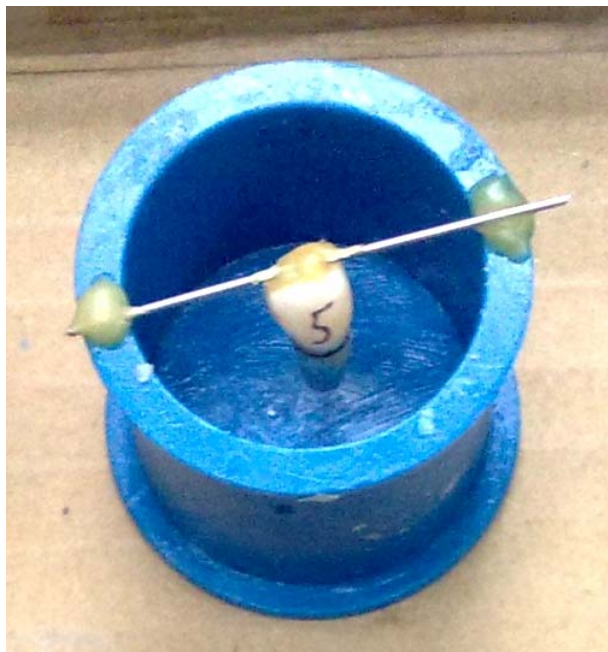
Figure 1. The tooth inside plastic mould ready to be embedded in resin.
