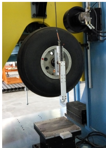
Figure 3: Landing gear drop test apparatus (Hidayat, Istiyanto, Sumarsono, & Marta, 2017)
