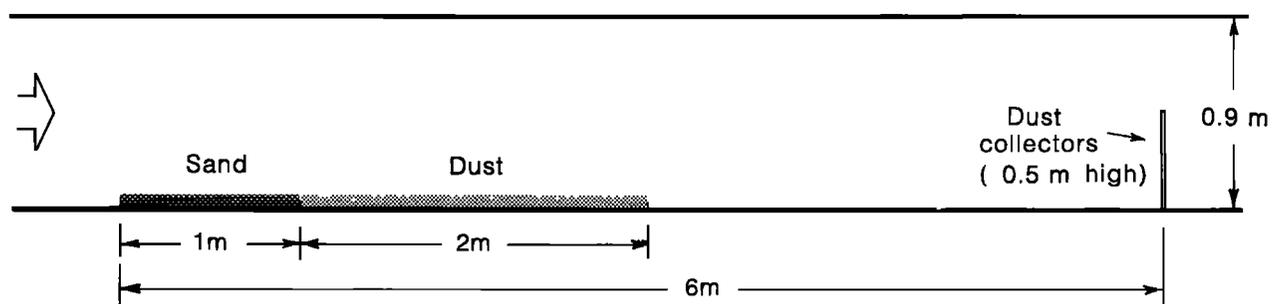
Fig. 1. Schematic illustration of the principal experimental ("bombardment") configuration.
