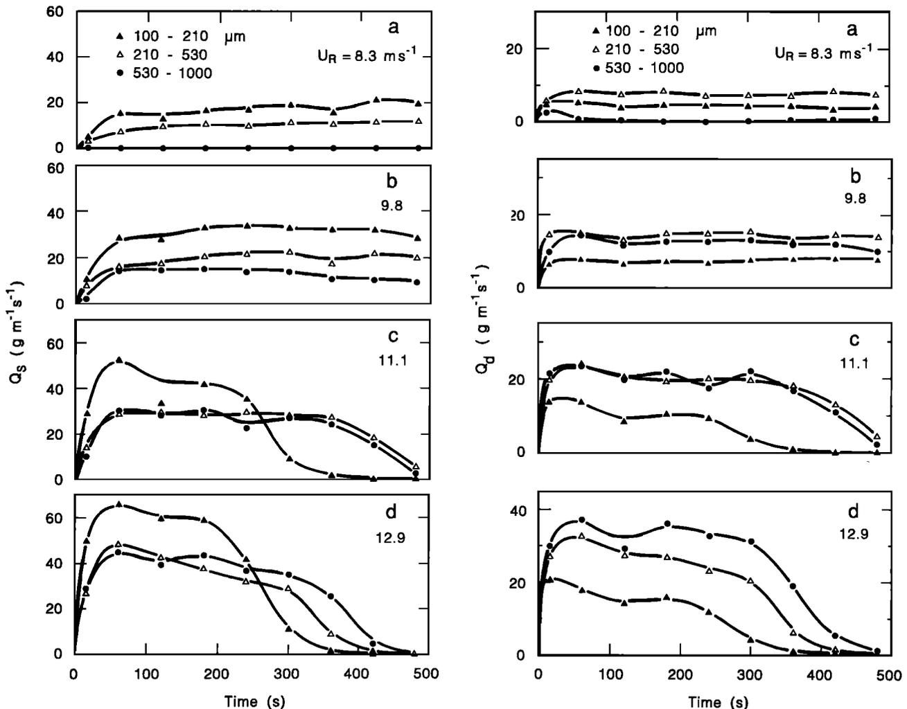
Fig. 5. Time evolution of (a) streamwise sand flux,  $Q_s$ , (b) streamwise dust flux,  $Q_d$ , and (c) the ratio  $Q_d/Q_s$  for three saltation size classes at four reference wind speeds,  $U_R$ .
