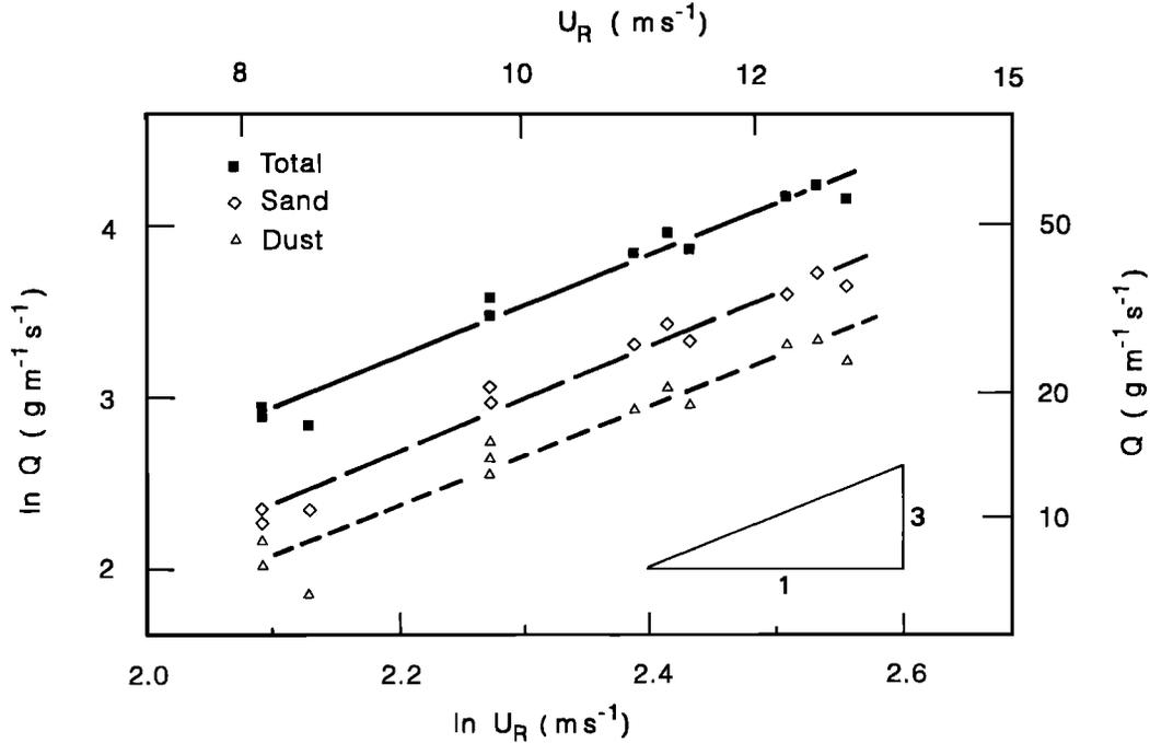
Fig. 4. Streamwise fluxes of sand,  $Q_s$ , dust,  $Q_d$ , and total mass,  $Q_t$ , for the 210 to 530- $\mu\text{m}$  saltation size class, plotted against reference wind speed,  $U_R$ , in logarithmic coordinates.
