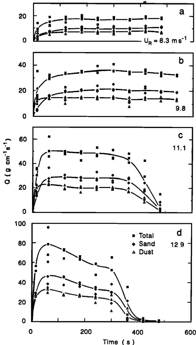
Fig. 3. Time evolution of streamwise fluxes of sand,  $Q_s$ , dust,  $Q_d$ , and total mass,  $Q_t$ , for four reference wind speeds, in the "bombardment" configuration. Saltation size class is 210 to 530  $\mu\text{m}$ .
