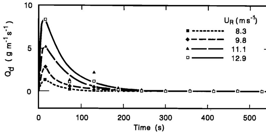
Fig. 2. Decay of streamwise dust flux,  $Q_d$ , with time for four reference wind speeds,  $U_R$ , in the "pure dust" configuration.
