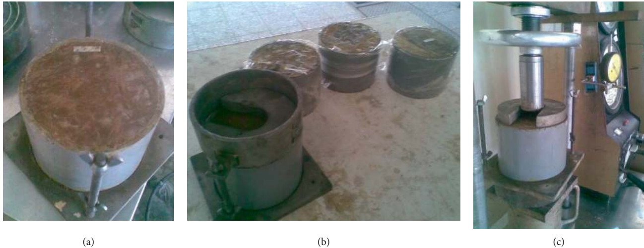
FIGURE 4: California bearing ratio test: (a) mould, (b) samples after 7 days of curing, and (c) California bearing ratio test apparatus.
