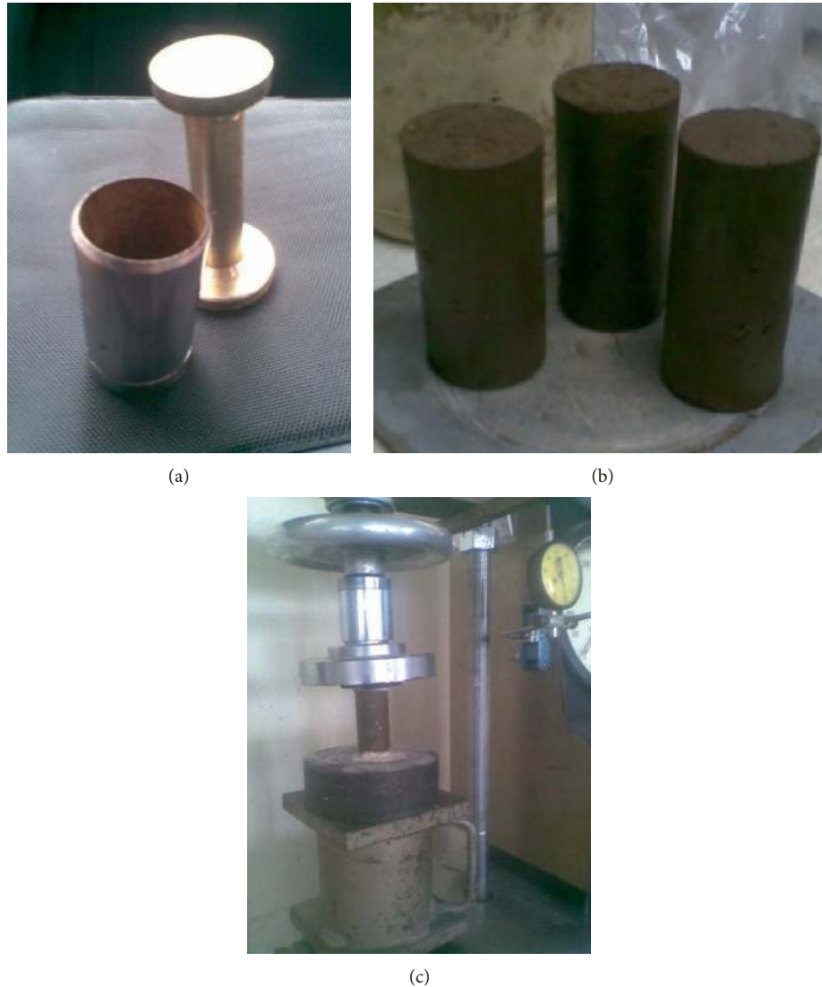
FIGURE 3: Unconfined compressive strength test: (a) mould, (b) prepared samples, and (c) sample under loading.
