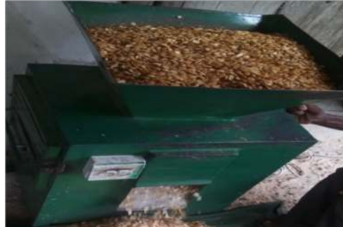
Plate 5: Improved Aba Melon Shelling Machine
