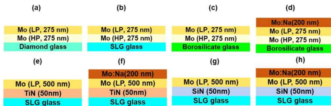
Figure 1. Different back contact designs used for CIGS solar cell fabrication: (a) Dia/Mo, (b) SLG/Mo, (c) Boro/Mo, (d) Boro/MoNa, (e) SLG/TiN/Mo, (f) SLG/TiN/MoNa, (g) SLG/SiN/Mo, and (h) SLG/SiN/MoNa.
