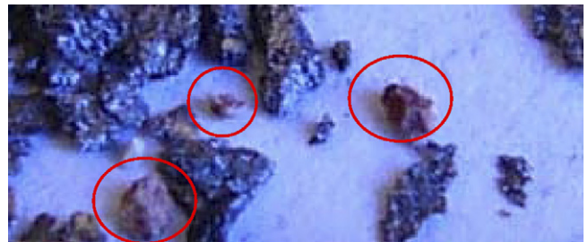
Fig. 14. Reddish fragments (typical size about 1 mm) observed among regular black scattered pieces after dynamic testing and comminution of C_{Pitch}/Al-Mg specimen bulk damaged at high-strain rate ( 5000\text{ s}^{-1} or 7000\text{ s}^{-1} ). (For interpretation of the references to color in this figure legend, the reader is referred to the web version of the article.)
