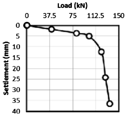
Figure (9) Load-Settlement relation of pile with D= 30 cm and L= 450 cm.
