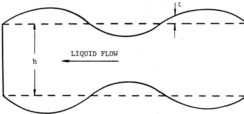
Fig. 10. Symmetric capillary waves in a thin film.
