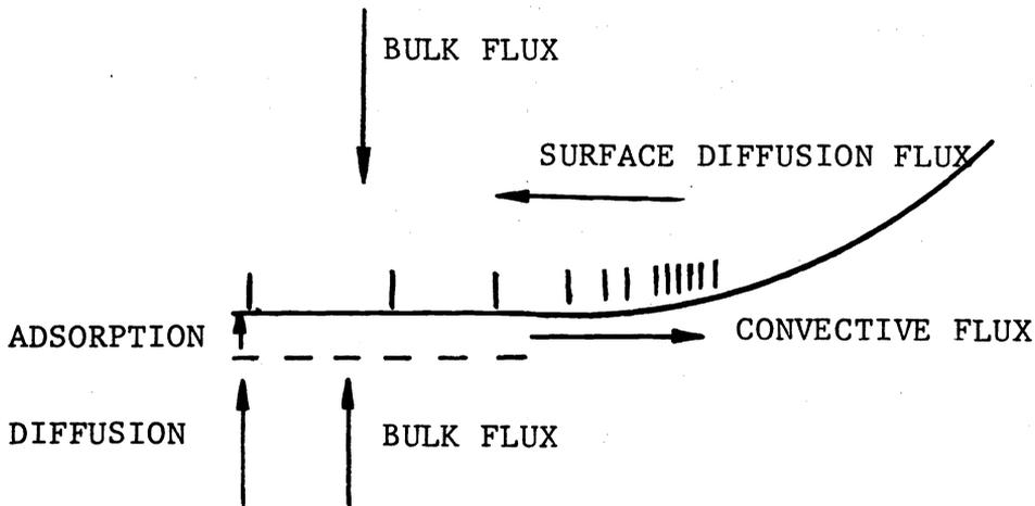
Fig. 2. Surfactant mass balance at the film surface.
