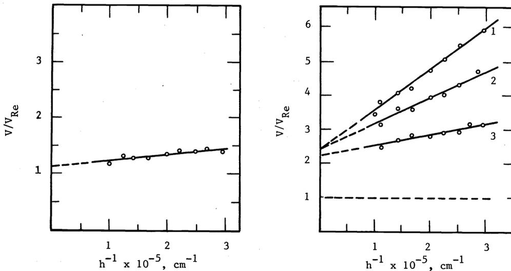
Fig. 7.  $V/V_{Re}$  vs.  $h^{-1}$  for nitrobenzene films: (a) surfactant silicon oil,  $2.78 \times 10^{-5} \text{ M}$ ; (b) surfactant  $C_{12}H_{25}OH$ : (1)  $1.1 \times 10^{-2} \text{ M}$ ; (2)  $4.4 \times 10^{-2} \text{ M}$ ; (3)  $17.8 \times 10^{-2} \text{ M}$  (Ref. 33).
