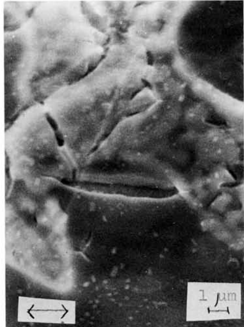
FIG 3.—Scanning electron micrograph of longitudinal section of tensile bar pulled to failure. Arrow, tensile direction.
