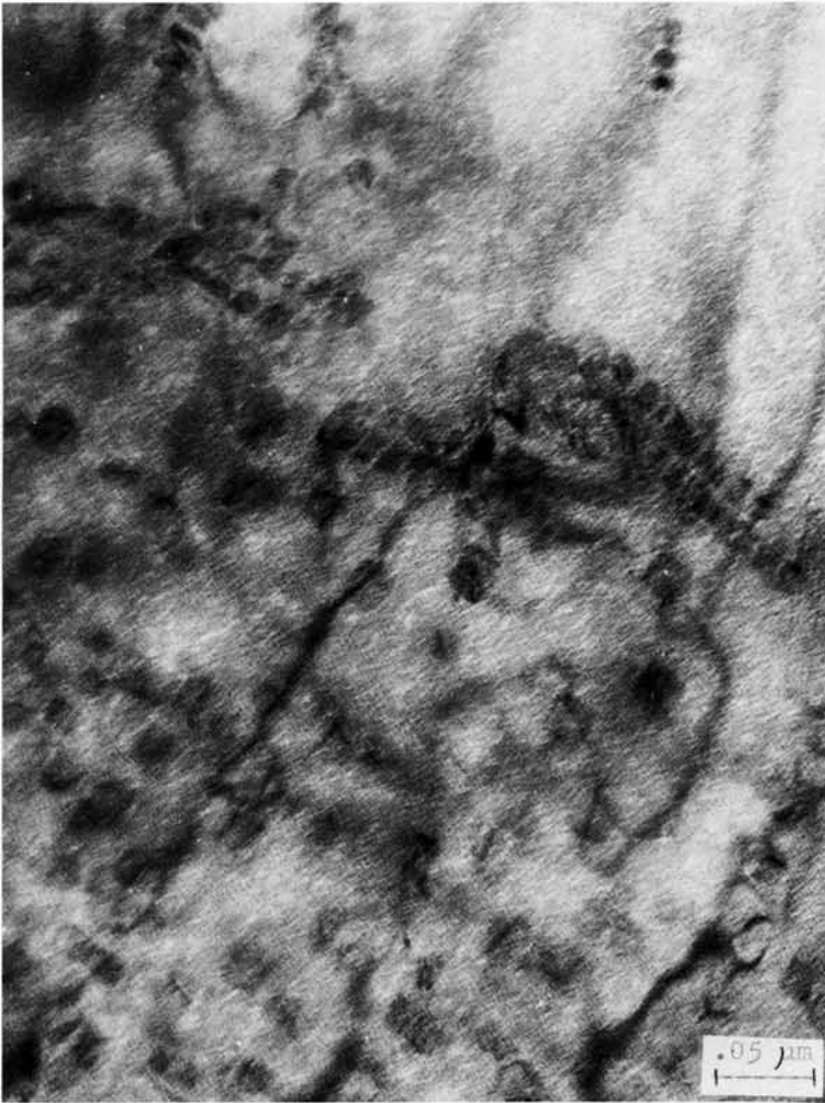
FIG 9.—Transmission electron micrograph of (130) \alpha phase and \alpha - \text{Co}_3\text{Ta} in heat-treated 9.1% Ta alloy.
