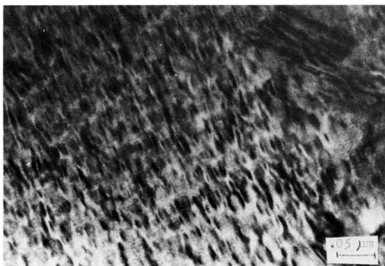
FIG 7.—Transmission electron micrograph of (100) ordered \alpha phase and \alpha -Co 3 Ta in 13.8% Ta alloy.
