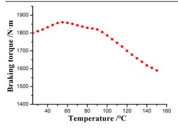
Figure 9. Curve of the temperature and the braking torque.
