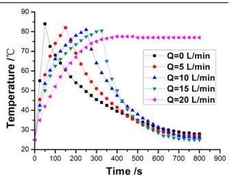
**Figure 11.** Curves of the temperature in terms of time at different cooling water flow rates
