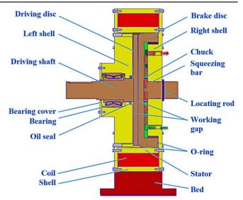
Figure 4. Basic structure of the high-torque squeezing MRF brake.
