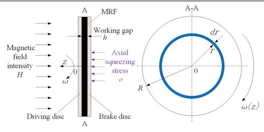
Figure 1. Working principle of the disc squeezing MRF brake.
