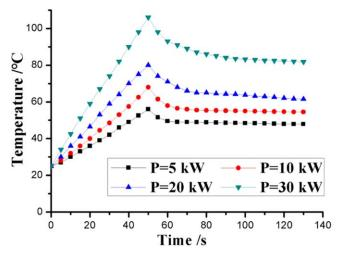
Figure 10. Curves of the temperature in terms of time at different slip powers.
