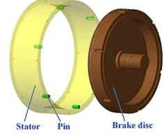
Figure 5. Brake disc assembly.
