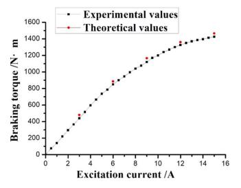
Figure 7. Curves of braking torque and excitation current
