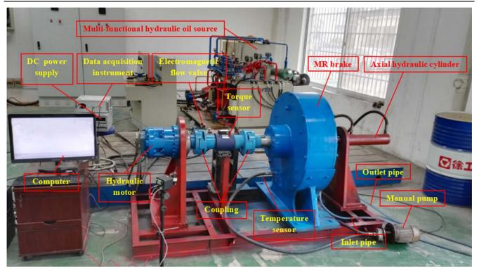
Figure 6. Temperature-torque performance experimental system.
