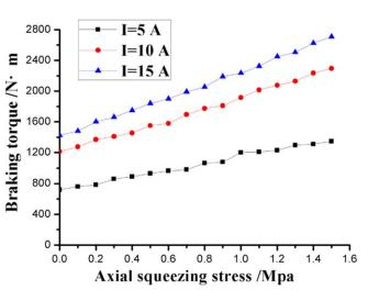
**Figure 8.** Curves of the braking torque and the axial squeezing stress at different excitation currents.
