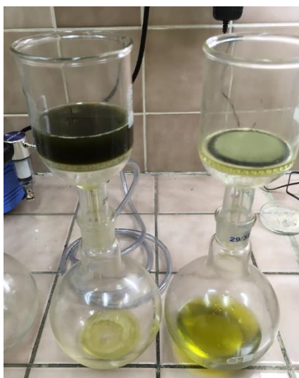
Figure 6. Separation of bleaching earth from oil.
