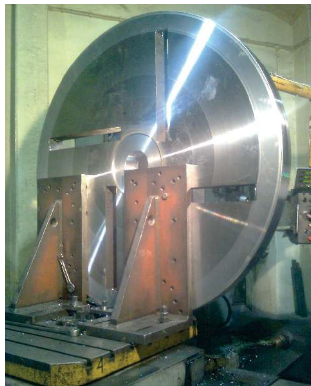
Figure 4 Boring holes in the disc chipper
