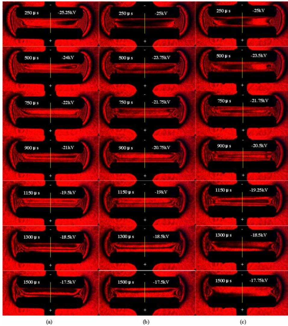
FIG. 3. The electro-optical field of propylene carbonate of the different electrode materials: (a) aluminum; (b) copper; (c) stainless steel.
