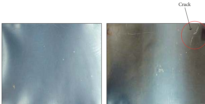
FIGURE 2: Oxo-degradable LDPE films at 0 and 330 hours of UV exposure in a Xenon arc chamber.
