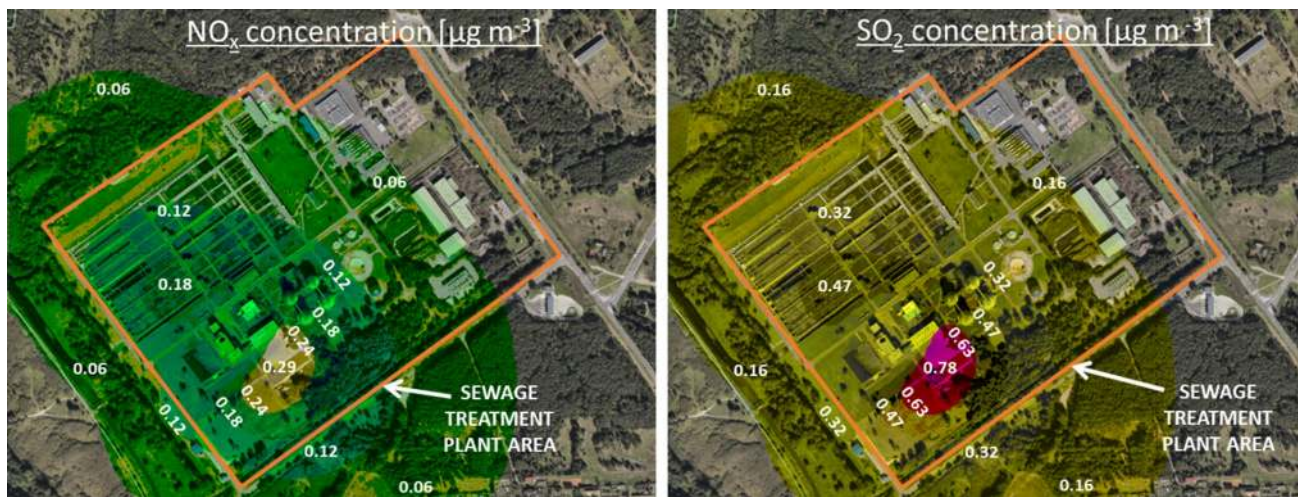
Fig. 4 Average annual concentration of NO x and SO 2 emitted from the analyzed system
