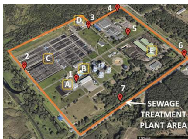
Fig. 1 Location of measurement points (1–7) in GOS–ŁAM, including the thermal sludge transformation system a , boiler and power plant b , sludge chamber c , inlet chamber and screen room d and the composting facility e Source: Google Maps
