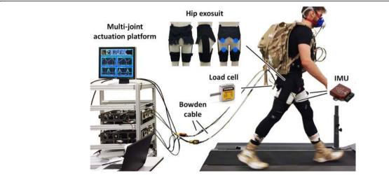
Fig. 1 Experimental setup with a participant wearing a soft exosuit that assists hip extension via Bowden cable. The assistive force is transmitted from the multi-joint actuation platform (on the left) to the wearer
