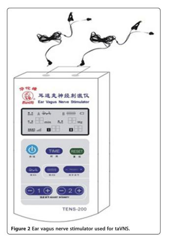
taVNS groups were 1 mA of electrical current at a frequency of 20 Hz with pulse duration  $\leq$  1 ms, administered twice daily. The intensity was adjusted based on the individual tolerance of patients. Each postprandial treatment lasted 20 minutes and was applied half of an hour after eating. After the training session, all subsequent treatments were applied independently by the patient at home.
