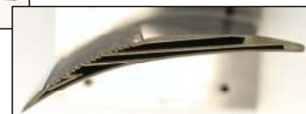
Figure 7. Details of Soft Vane acoustic treatment design; leading edge of vane is on the left.
