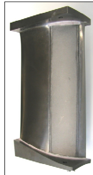
Figure 6. Acoustically treated Soft Vanes (SV), forward looking aft.
