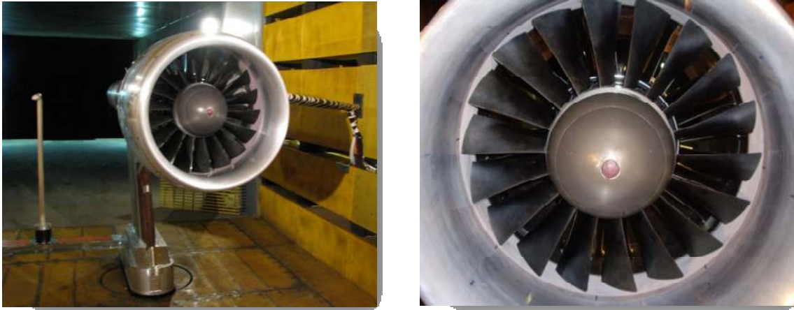
Figure 1. Ultra High Bypass fan model hardware installed in the NASA Glenn 9’x15’ LSWT.
