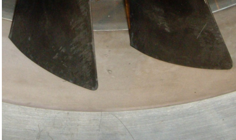
Figure 5. Baseline hardwall (HW) fan case rubstrip.
