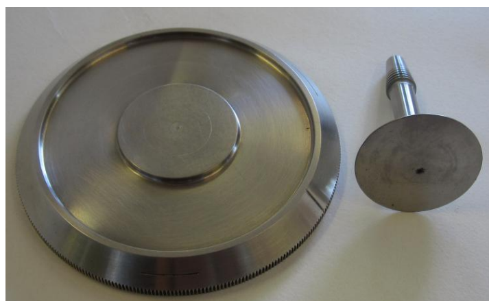
Figure 5.15. Cone-plate sensor geometry used for the hysteresis loop and shear rate step tests.
