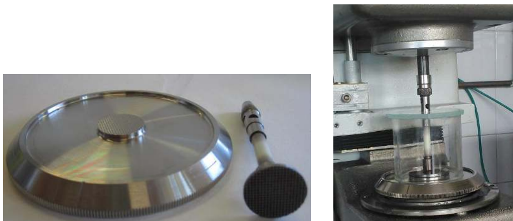
Figure 5.14. Serrated plate-plate sensor geometry used for the creep test (on the left) and isolation system (on the right).
