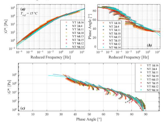
**Figure 5.** Comparison of master curves of complex shear modulus (**a**), phase angle (**b**), and black diagram (**c**) for 160/220\_I.
