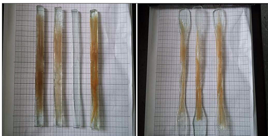
Fig. 2. Flexural and tensile test specimens
