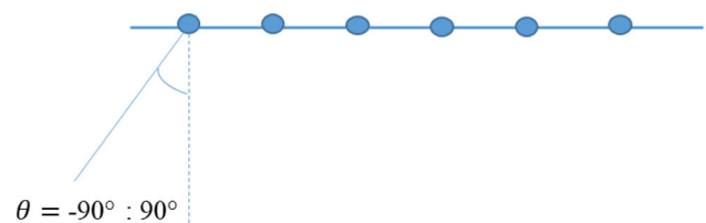
Fig. 1 Sketch of the angle of the critical plane on one point.
