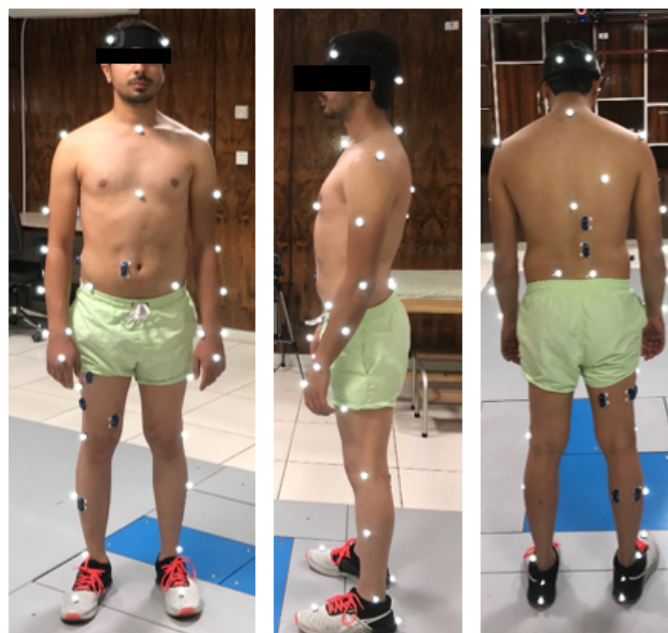
Figure 1. Experimental setup used for GAIT measurements. The motion analysis lab for kinematics and kinetics measurements in Movafaghian (Sharif University of Technology, Tehran, Iran) consists of high-speed motion captures and force plates.
