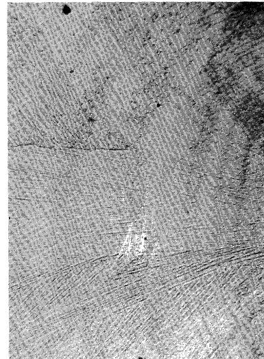
Photo. 2. An example of stray crystal which originated in the weld metal of 1050 aluminum ( \times 42 )
