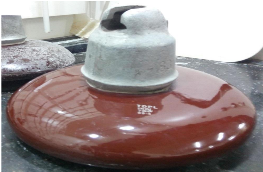
Fig. 8: Uncoated Insulator Post Insulator Bushing of 70kN from Tehri Distribution Power Limited, Power Transmission Corporation of Uttarakhand Limited.
