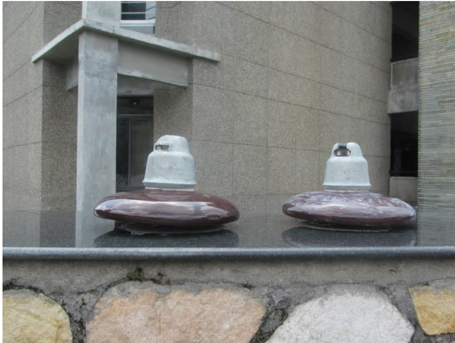
Fig. 11: Coated and Uncoated Insulator Is Kept for Observation in a Commercial Building Construction Polluted Area.
