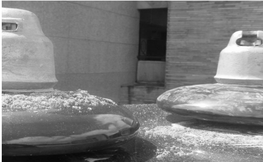
Fig. 14 (B): Left Image in the Figure: Uncoated Insulator with Deposition of Mist and Dust Still on The Surface. Right Image in the Figure: Coated Insulator with All the Deposition of Mist and Dust Roll off from the Surface of the Insulator when Both the Insulator Kept at Same Location.
