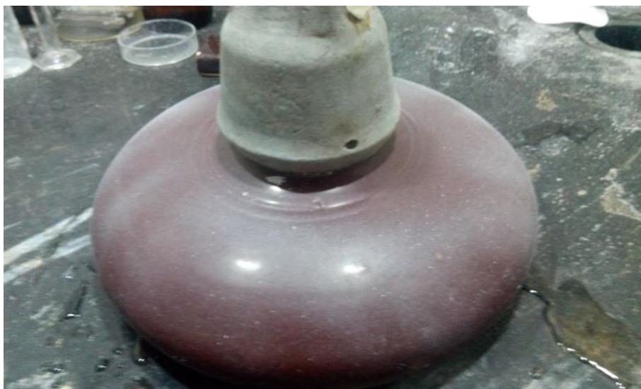
Fig. 12 (B): Coated Insulator without Any Dust Particle.
