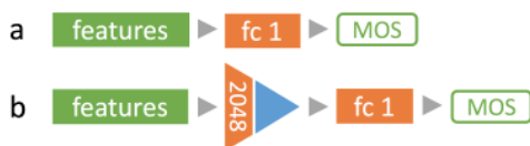
Figure 4: a) Single-1FC architecture, b) Single-3FC with X = 2048 . Complete feature learning architectures used to train on narrow MLSP features ( 1 \times 1 \times b ). For each architecture we predict the mean opinion scores (MOS).
