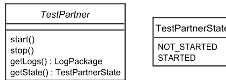
Figure 5.5.: The Lifecycle and Interface of the Test Partner
