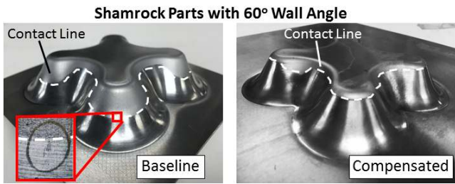
Fig. 10. Compensated toolpath maintains better contact. Strains were measured from a laser marked circle grid.
