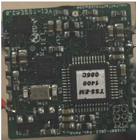
FIGURE 5: Gesture sensor including 3-axis gyroscope, accelerometer, and magnetometer and reference Euler angles.
