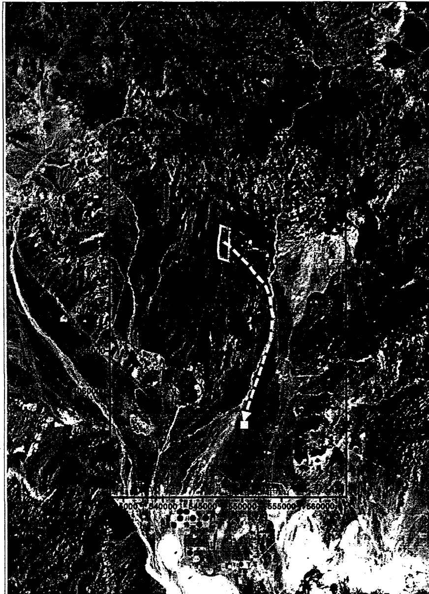
Figure 1. Region near the potential waste repository at Yucca Mountain, Nevada. The base map is a false-color infrared satellite image. The outline of the potential repository is shown with the light bold line. The inferred flow pathway in the saturated zone from beneath the repository to a hypothetical receptor at a distance of 20 km is shown by the dashed line. The locations of wells at which water level measurements have been made are shown by the + symbols. The outlined area is 30 km by 45 km, with the axes labeled in UTM coordinates (meters).
