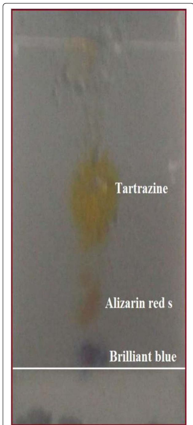
Fig. 6 Separation achieved separation (or resolution) of three-component mixture of dyes (tartrazine, alizarin red S and brilliant blue) on Pani@SIG-ES layer developed with M_3 mobile phase
