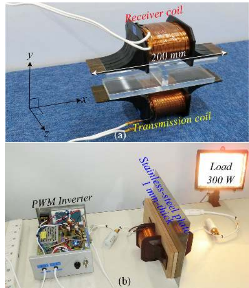
Fig. 3. Prototype P6 used in simulation: (a) Photograph of coils, (b) Demonstration of WPT through a stainless-steel plate (UNS S30400). When driven at 400 Hz, 80% efficiency and 317 W output were achieved when transmitting power through a 1 mm-thick UNS S30400 plate over a distance of 30 mm
