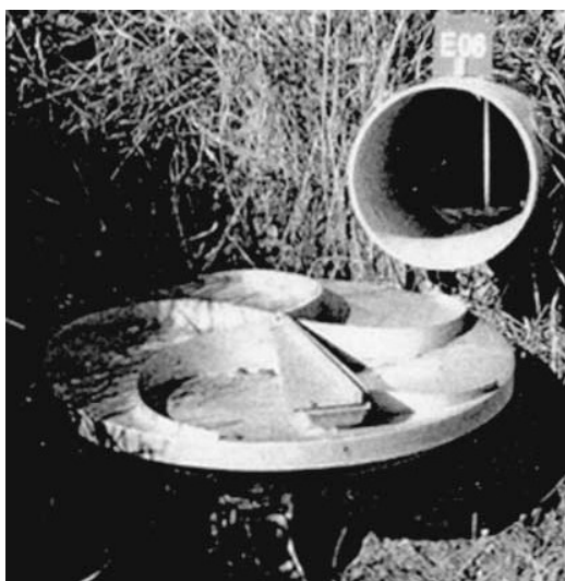
Fig. 3. Coshocton-type wheel runoff sampler at the Scheyern Experimental Farm.
