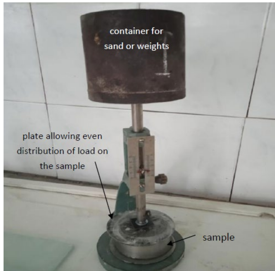
Figure 2. Device for determining the structural strength.
