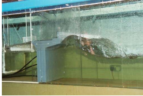
Figure 10. Example of a wave being deflected seaward in the promenade wall study
