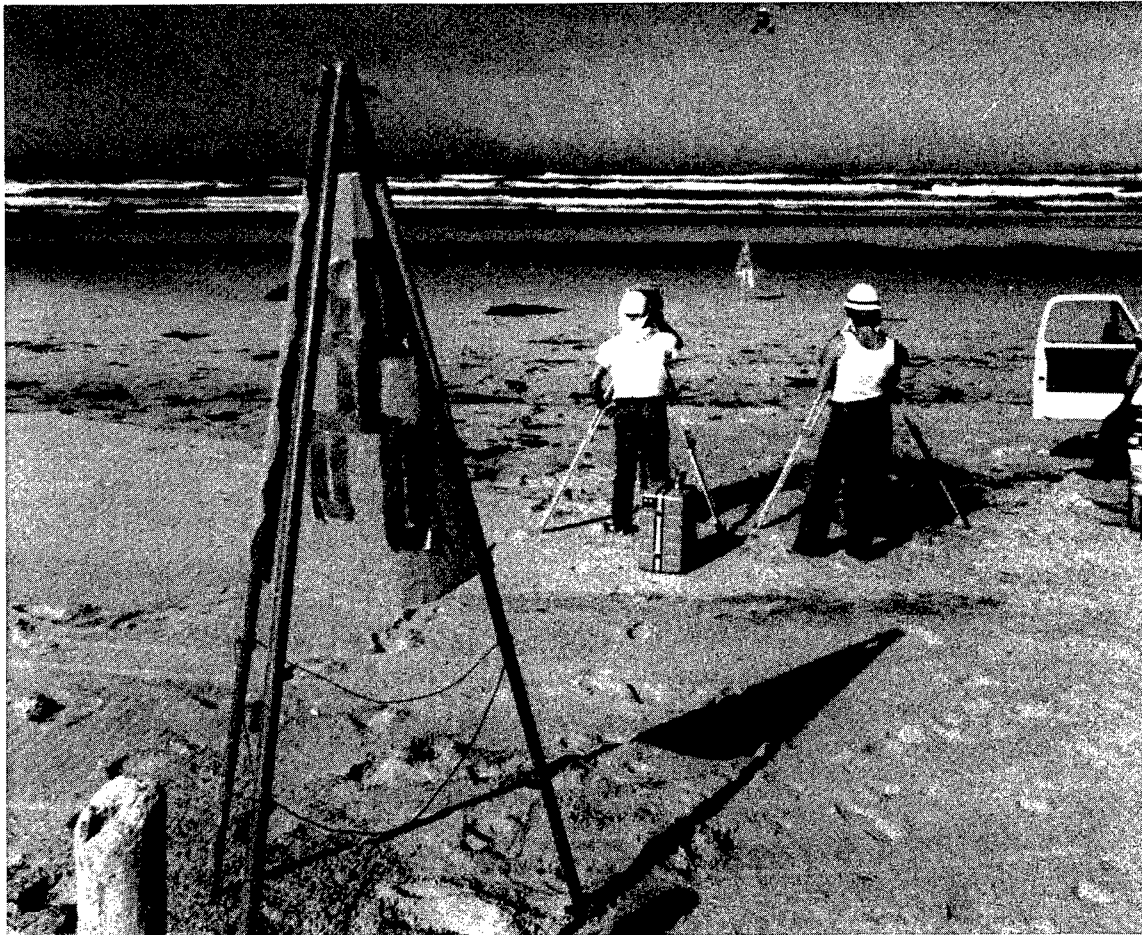
Figure 33. Helicopter, range poles, and total station on profile line
