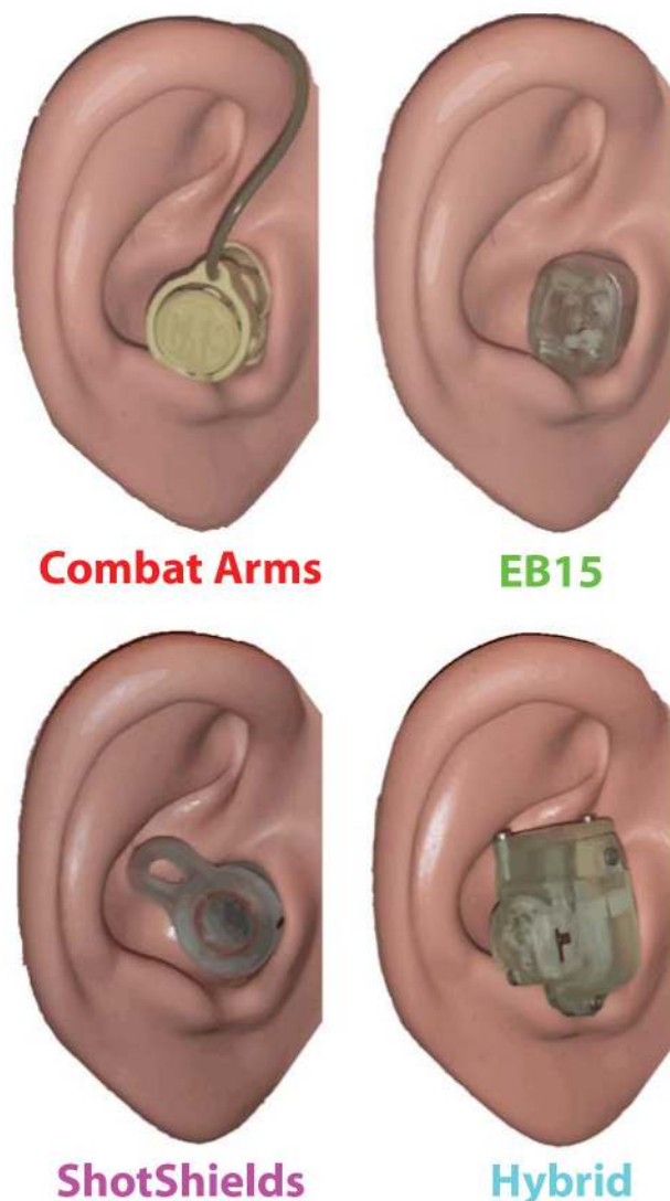
Fig 1. Hearing protection devices (HPDs) tested in the current study. Four HPDs are illustrated as worn inside the right ear of a test manikin (G.R.A.S. 45CB Acoustic Test Fixture).
