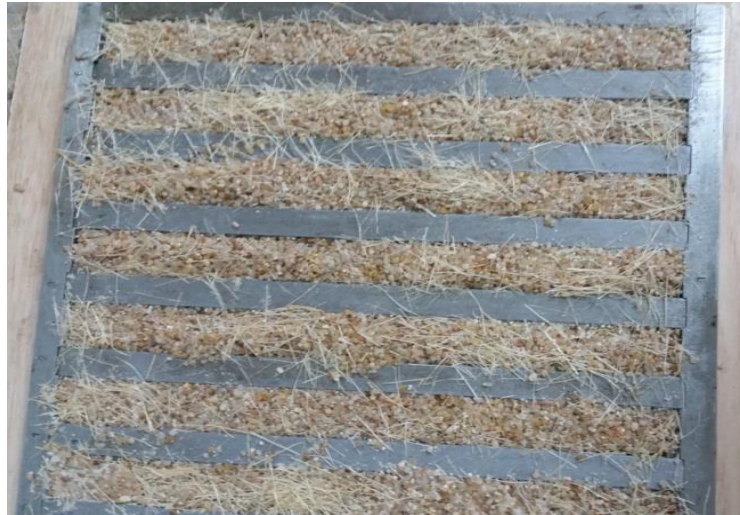
Fig 1. Mould filled with PCS may contain seven specimens.
