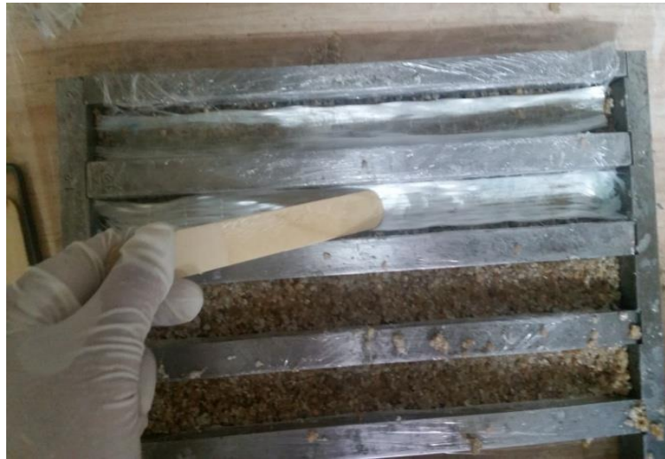
Fig 2. Filling of mould with the glass fibre band incorporations.
